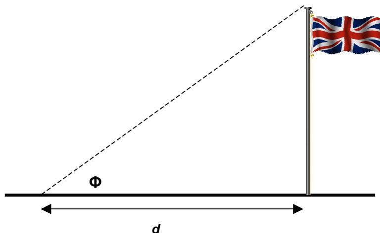
3.34 If the uncertainty in  $d$  is, say,  $\pm 0.1$  m then the estimate of  $h$  could be anywhere between  $(7.0 - 0.1) \tan(37)$  and  $(7.0 + 0.1) \tan(37)$ , i.e. between 5.200 m and 5.350 m. A change of  $\pm 0.1$  m in the input quantity  $x_i$  has resulted in a change of  $\pm 0.075$  m in the output estimate  $y$ . The sensitivity coefficient is therefore  $\frac{0.075}{0.1} = 0.75$ .
